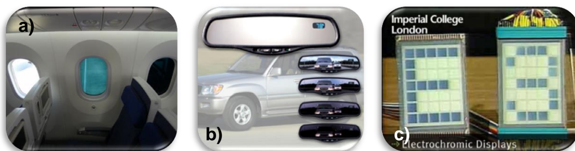
Figure 1.2 - Three main applications for EC materials in ECDs: a) smart windows,[76] b) rear mirrors [77] and c) PM displays.[77]
