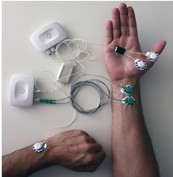
Figure 3.3: Electrode positioning. Stimulation electrodes are placed on the right wrist (anode on top). Ground electrode is placed on the opposite wrist. Acquisition electrodes are placed on the muscle surface of the thumb.
