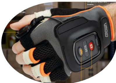
Figura 6. 5 - Luva com controlo remoto Adaptado de: Crown Equipment Corporation (2013b)
