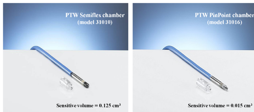
FIGURE 2.17: PTW Semiflex ionization chamber of 0.125 \text{ cm}^3 , on the left; and PTW PinPont chamber of 0.015 \text{ cm}^3 on the right side. Images from www.ptw.de
