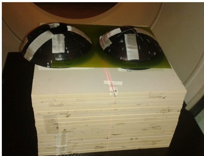
FIGURE 5.2: The NAOMI phantom. Left homogeneous breast and right breast with a hole placed on top of a set of water-equivalent slabs to perform the measurements by placing an EBT2 film within two slices of the phantom.
