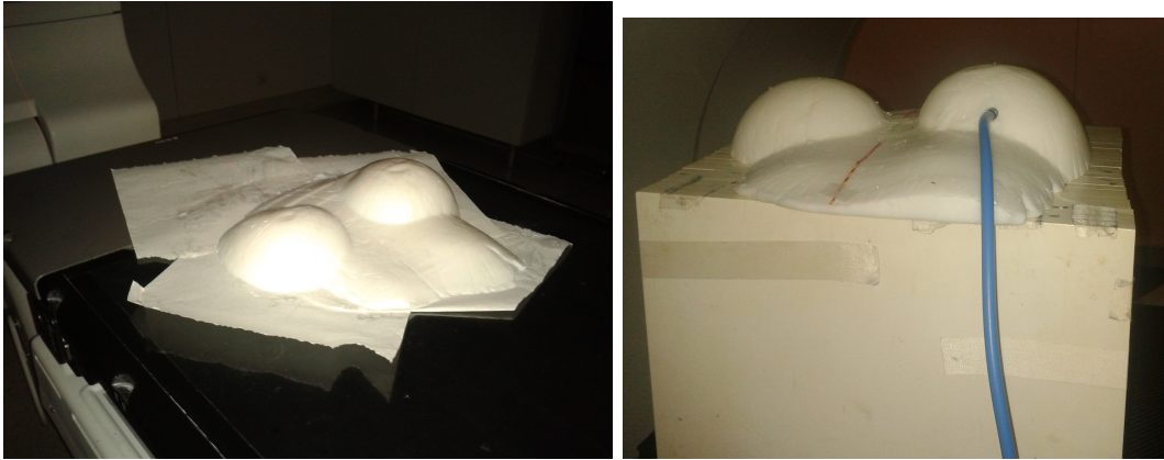
FIGURE 5.1: The Belem phantom. On the left, the breasts made of vegetal fat; on the right, the breasts are placed on top of a set of water-equivalent slabs to perform the measurements.
