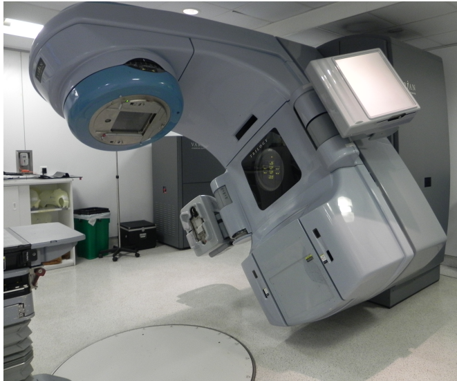
FIGURE 2.1: Example of a linac used in radiotherapy departments for clinical use.
