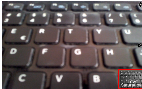
Figure 3.8: Frame detected as containing low saturation. Indicator is shown on the bottom right corner, which is the input frame converted into grayscale and in a reduced scale.
