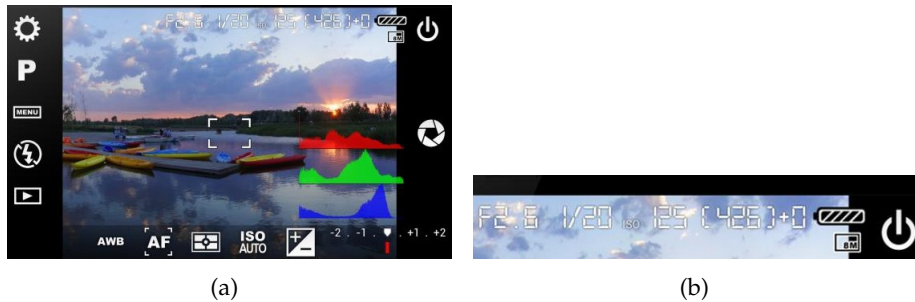
Figure 2.7: Camera FV5 interface (a) and indicators (b) of aperture, exposure time, ISO, etc [Vaz].
