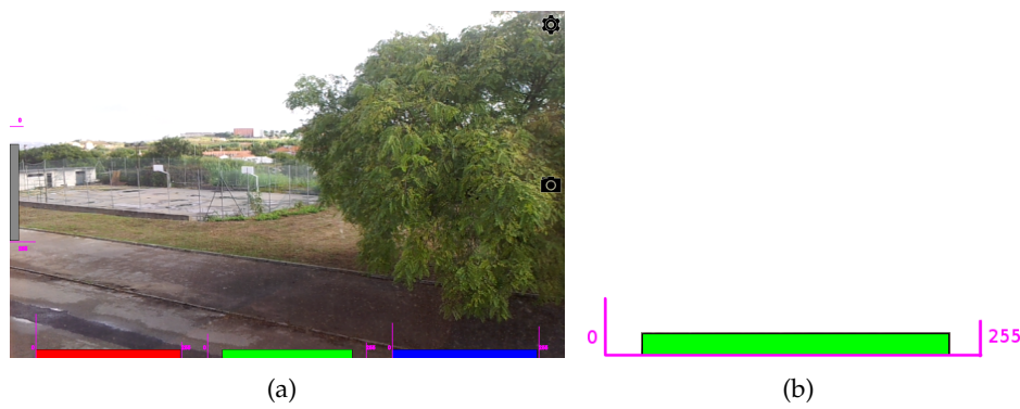
Figure 3.6: Visual cue chosen for the first implementation of the histogram being applied to a real-time scenario (a) and a reconstruction of the histogram made for the green channel that indicates de colour range in use and the amount of pixels near the limits (b).
