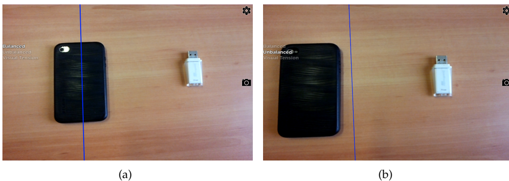
Figure 3.25: Examples of an unbalanced image with objects of different sizes where one is classified as unbalanced (a) and the other as balanced (b), as a result of the calculated symmetry axis.
