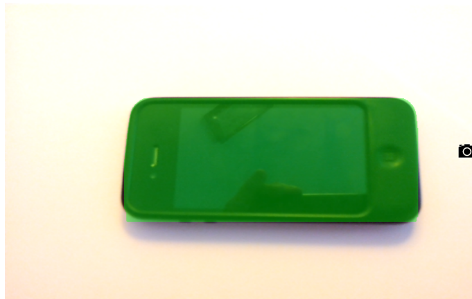
Figure 3.13: Example of object segmentation interface. The resulting mask of the algorithm is then displayed as a green overlay in the camera live feed.
