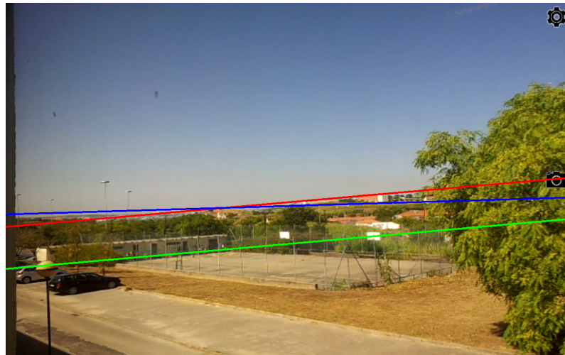
Figure 3.21: Example of horizon detection where the green and blue line are the result of the edge and color detector respectively. The red line represents the result of combining both methods.
