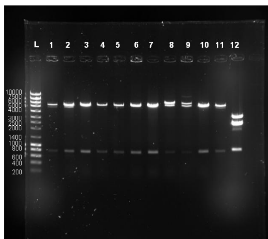
Figure 3.5 Evaluation of the hydrolysis of pAP001 of twelve selected colonies obtained from the subcloning procedure with restriction enzymes Nhe I and Eco R I by agarose gel electrophoresis (0.8 % (w/v) agarose). A volume of 2 \mu l of each reaction was applied. The positive clones were identified by the presence of a fragment with 843 bp.
