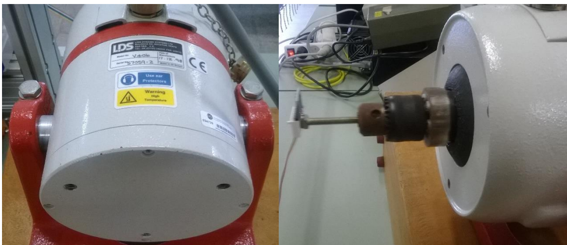
Figure 7 - Permanent Magnet Shaker. Sensor fixated to the Shaker moving axis (Right picture).
