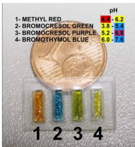
Figure III. 4 – Ionogel based wearable pH sensor for the analysis of human sweat [141]
