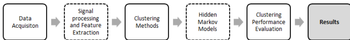
Figure 1: Overall structure of the framework developed for HAR systems. After the ACC data acquisition, the signal processing and the feature extraction stages are carried out and its results are used in clustering methods and in the HMM application. Finally, the clustering performance evaluation is applied. The hatched blocks show novel approaches for activity recognition.
