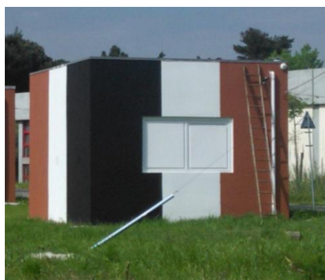
Figure 1. Full-scale experimental cell painted with three reflective paints.
