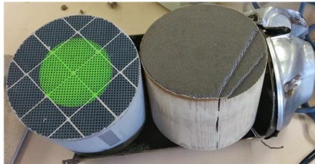
Figure 2.1- At left Diesel Particulate Filter (DPF) and at right Diesel Exhaust Catalyst (DOC)
