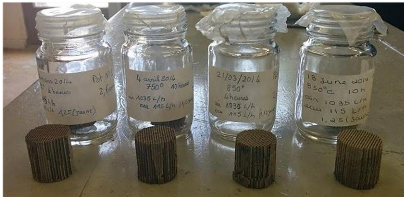
Figure 2.2 - Catalyst samples. From left to the right: DOC 750°C 4h, DOC 750°C 10h, DOC 850°C 4h and DOC 850°C 10h
