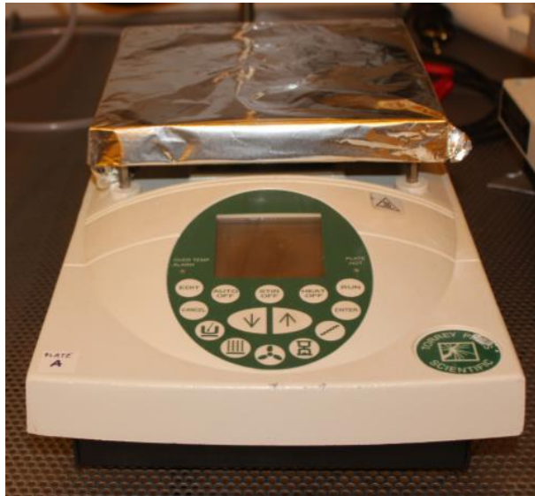
Figure 3.9. Picture of the hot plate used to perform thermal annealing of thin films and devices.
