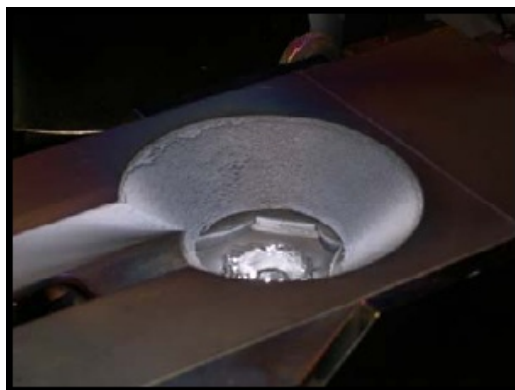
Figure 3.8. Picture of the electron beam evaporation crucible unit.
