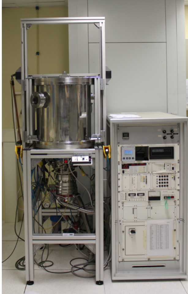
Figure 3.6. Picture of the electron beam deposition system existing at CEMOPs clean room at New University of Lisbon.
