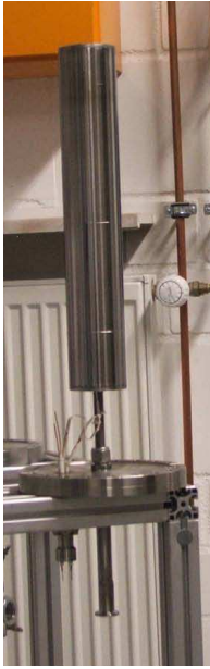
Figure 3.19: Assembled probe; section of a ASS tube where two steel covers (one flat and other with a hole where is welded a 12 mm diameter steel tube) are welded in both ends. The specimen is introduced in a CF blank flange, fixed recurring to a Swagelok squeeze connection and a sensor is wired at the middle of its length
