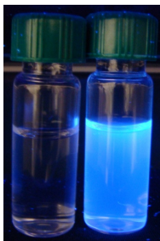
Figure 1.12 Left glass vial: pure water. Right glass vial: strong fluorescence phenomenon of PMetOx-DDA mw in aqueous solution under UV lamp.
