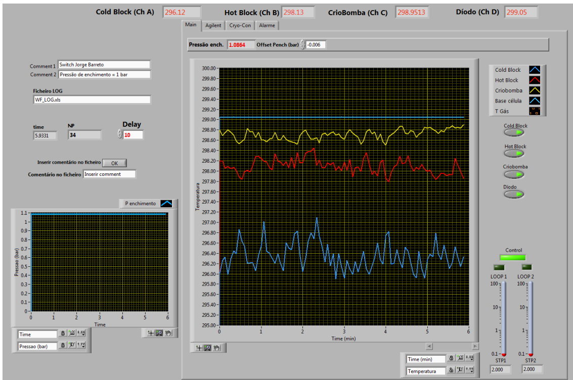
Figure 5.10: Main tab of the virtual instrument panel of the LabVIEW TM program used in this work. This tab includes the values of the temperature, pressure and LOOP 1 & 2. The remaining tabs allows to control the loops and hot block applied power.
