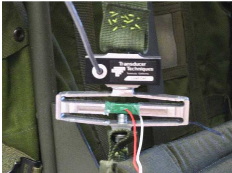
Fig. 2.14 Backpack energy harvester with mechanical amplification
