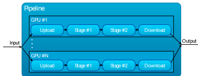
Figure 3.6: Pipeline skeleton execution (taken from [42])
