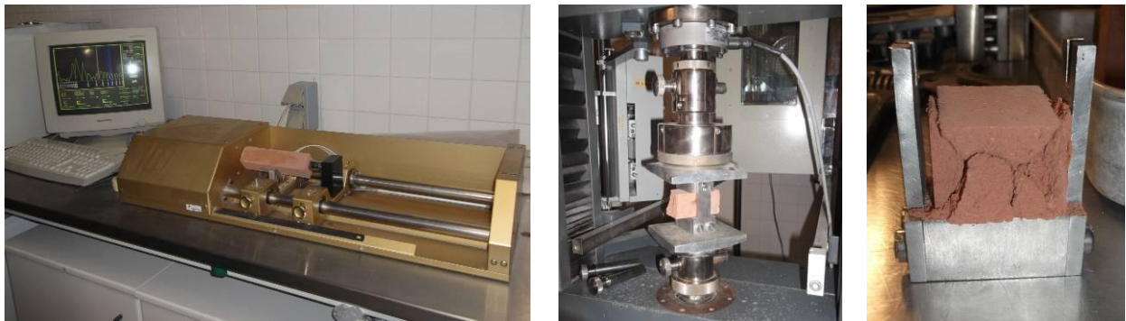
Figure 7. Sample being tested for dynamic modulus of elasticity (left) and for compressive test - being tested (middle) and conic fracture (right)
