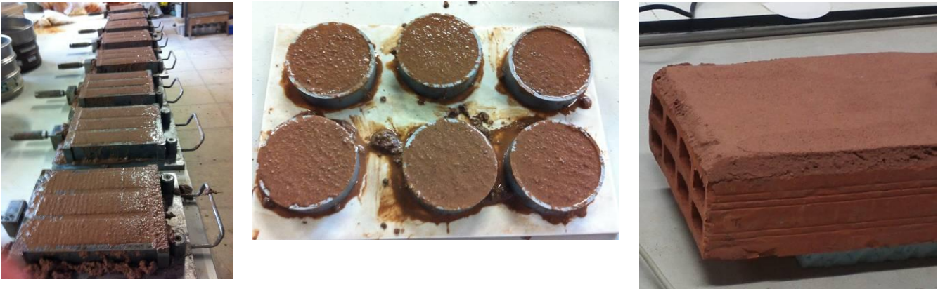
Figure 5. Prismatic (left), circular (middle) and on hollow brick mortar (right) samples
