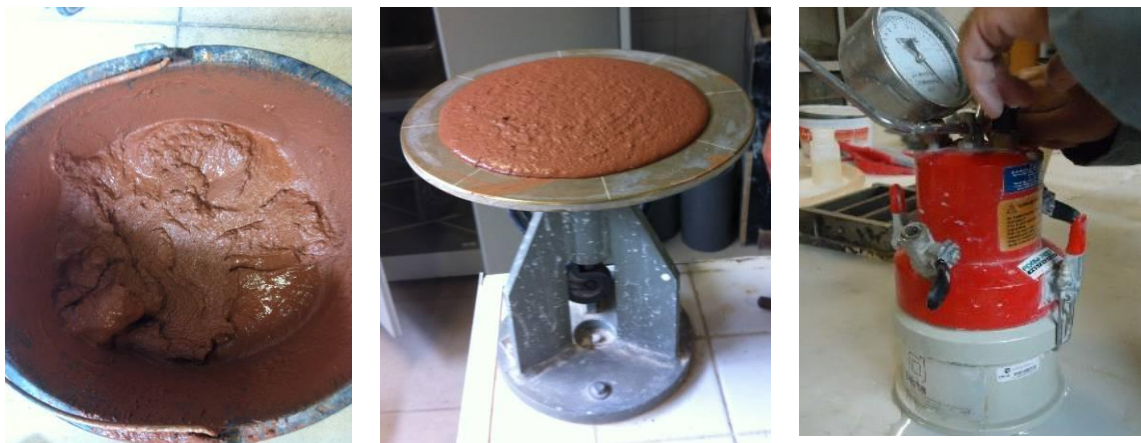
Figure 4. Fresh mortar (left), consistency flow table test (middle) and air content determination (right)
