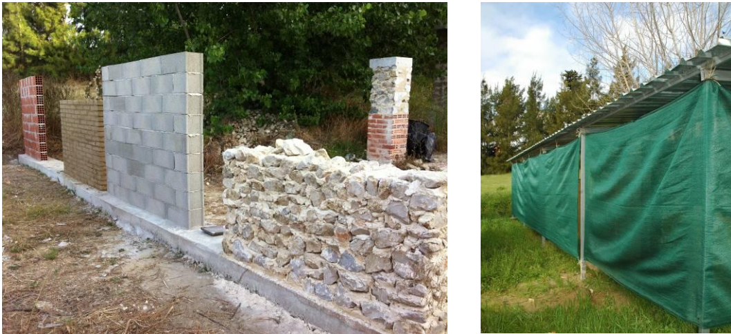
Figure 1. Four masonry test walls, yet unprotected – from the front to the back, rubble stone, concrete blocks, adobe and hollow bricks (left); protection of the experimental walls after plastered (right)
