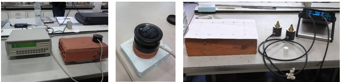
Figure 8. Mortar on brick (left) and circular samples (middle) being tested for thermal conductivity and equipment for ultra-sound determination (right)
