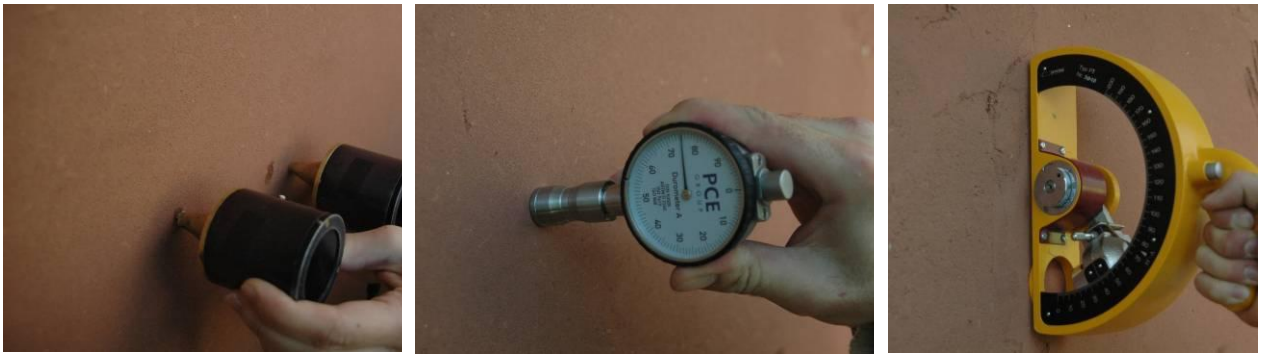
Figure 9. Ultra-sound (left), durometer (middle) and sclerometer (right) tests on plasters on the masonry test walls
