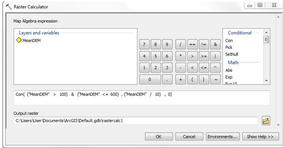
Figure 2.9 Raster calculator dialog box where a conditional (Con) function is used. MeanDEM as input Layer and map algebra expression where the desired operation is to divide all values between 100 and 600 inclusive of the input file by 10. All other values are assigned a value of 0.
