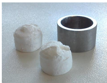
Figure 2.2 – Example of native CHT/PVA monoliths prepared by \text{scCO}_2 – assisted drying process.
