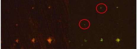
Fluorescence image showing bacterial distribution on a copper specimen under a triaxial permanent magnetic field. The image is split vertically. The left side shows orange and green spots, while the right side shows a higher density of green spots. Two red circles highlight specific green spots on the right side. |
