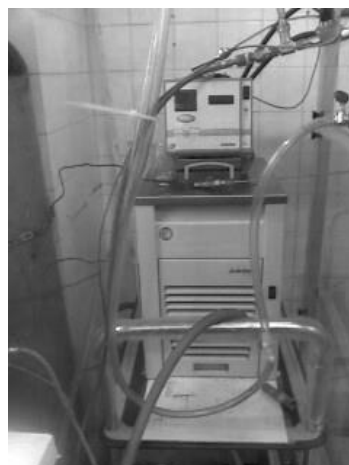
Figure C.6 - Thermostatic Bath, Refrigerator/Heater from Julabo.
