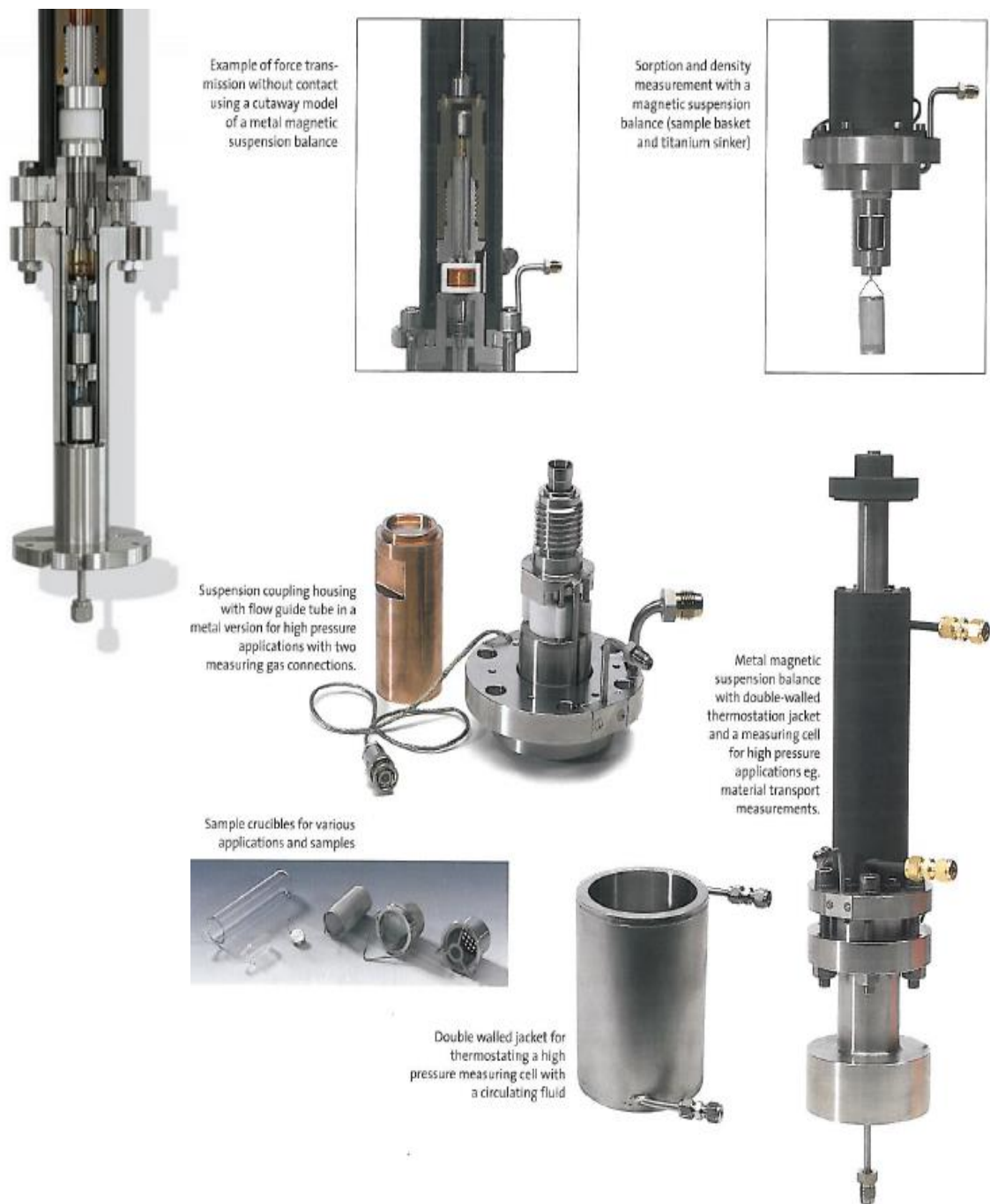
Figure 4.1 - Magnetic suspension balance components [60].
