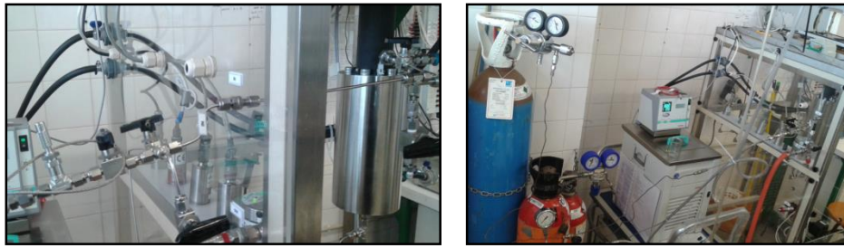
Figure 3.7: Inert, component and vacuum feed streams of the feed system unit.
