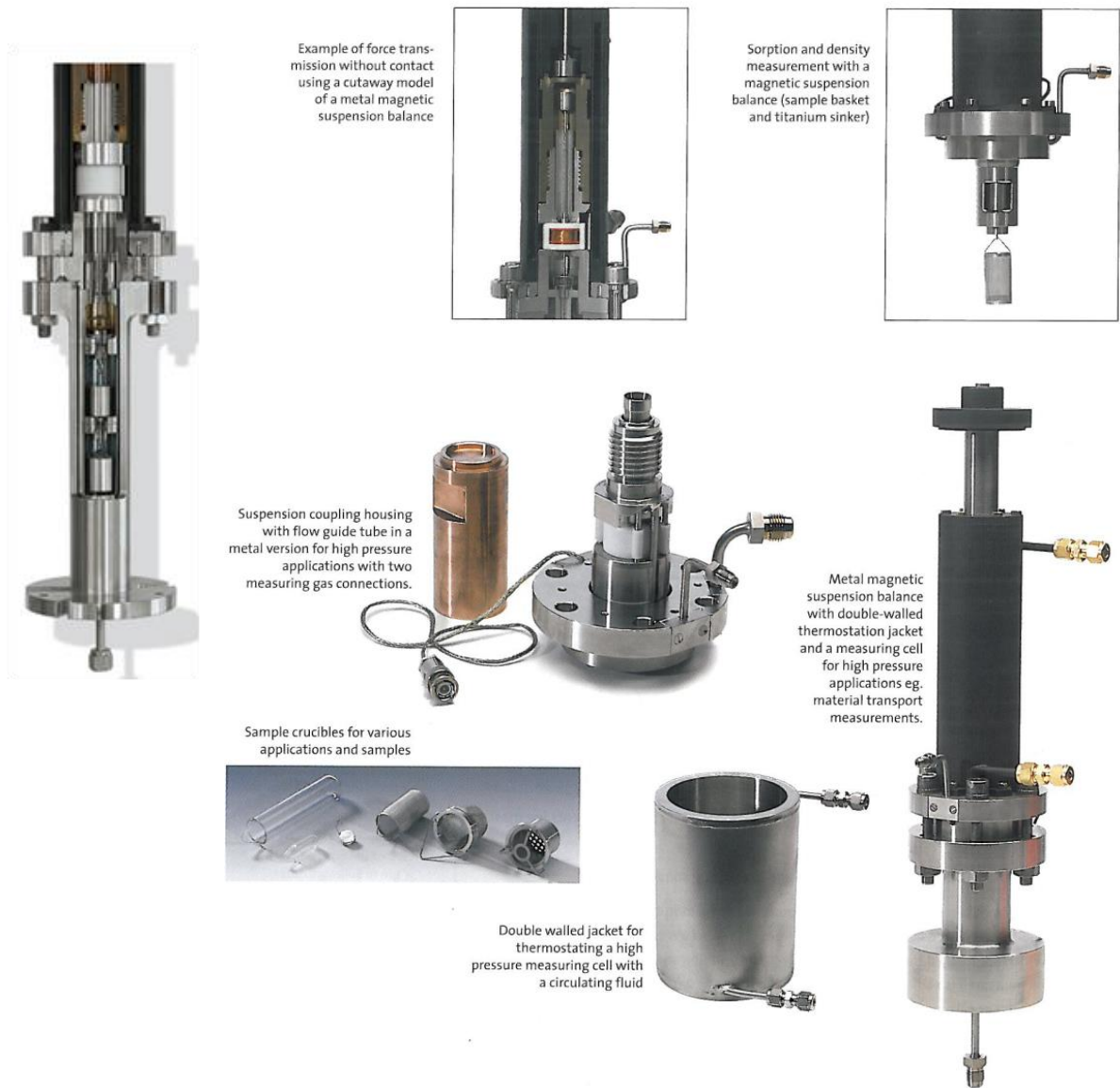
Figure 3.4: Magnetic Suspension Balance (MSB) components [58, 59].
