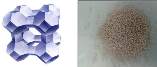
Figure 2.3: Typical Structure of zeolite type A (left) and image of the sample of zeolite 5A, used in the experimental work (right) [91].
