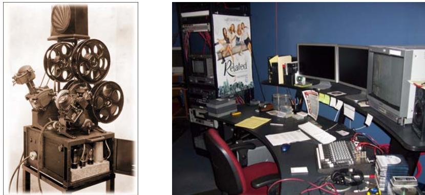
Figure 2.15: Film editing equipment: (a) Old Moviola machine for editing on film 20 . (b) Modern Editing Equipment 21 .
