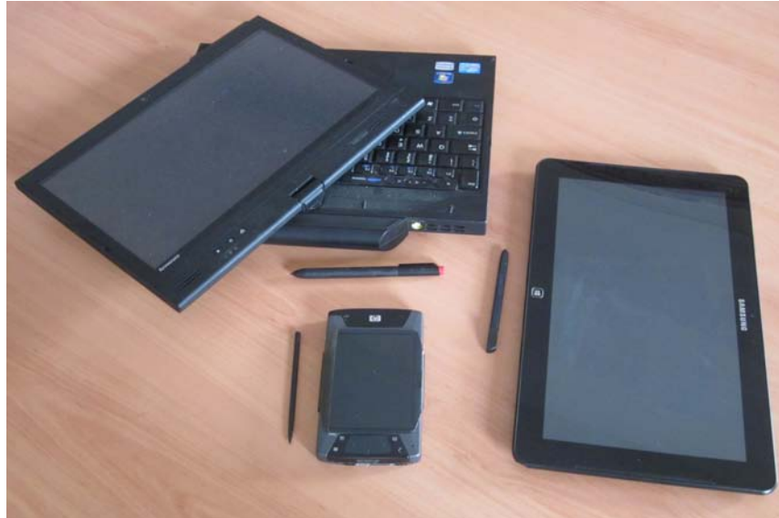
Figure 2.5: Tablet computers: a PDA on the left bottom, a convertible tablet on the left top and a tablet/slate computer on the right.
