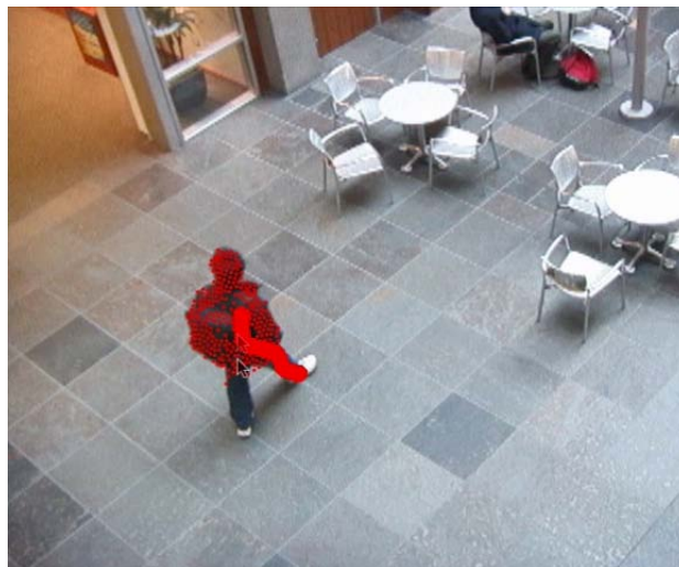
Figure 2.13: Selecting a region for tracking using point and group particles [GGCS08].
