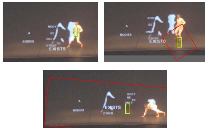
Figure 3.12: Tracking with CAMSHIFT: green ink strokes - annotation; yellow small rectangle - anchor; and the large red rectangle - CAMSHIFT's output 8 .
