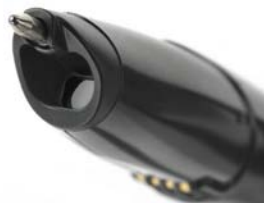
Figure 2.6: Anoto Pen: Regular ink pen and camera 11 .
