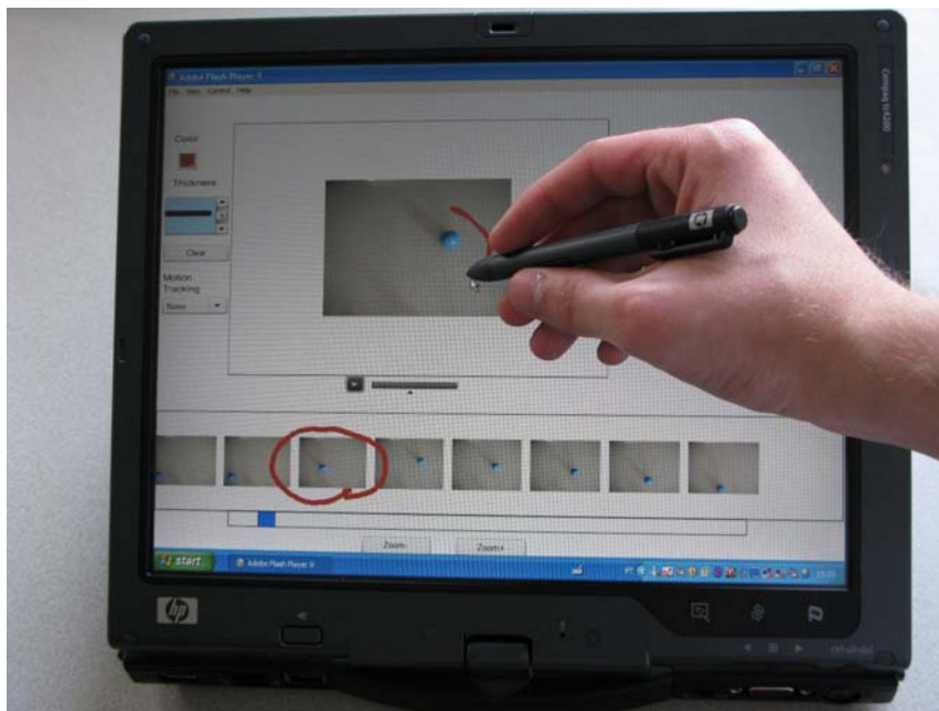
Figure 3.1: Pen-based video annotations: proof-of-concept prototype - annotating on a recorded video.
