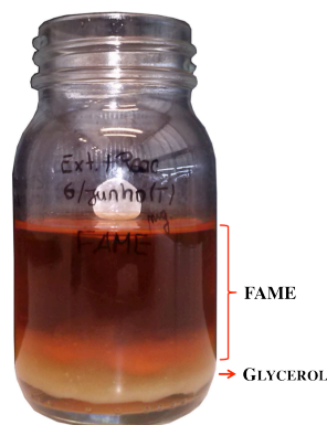
Figure 3.2.1 – Biodiesel produced in this work, from the extracted oil.
