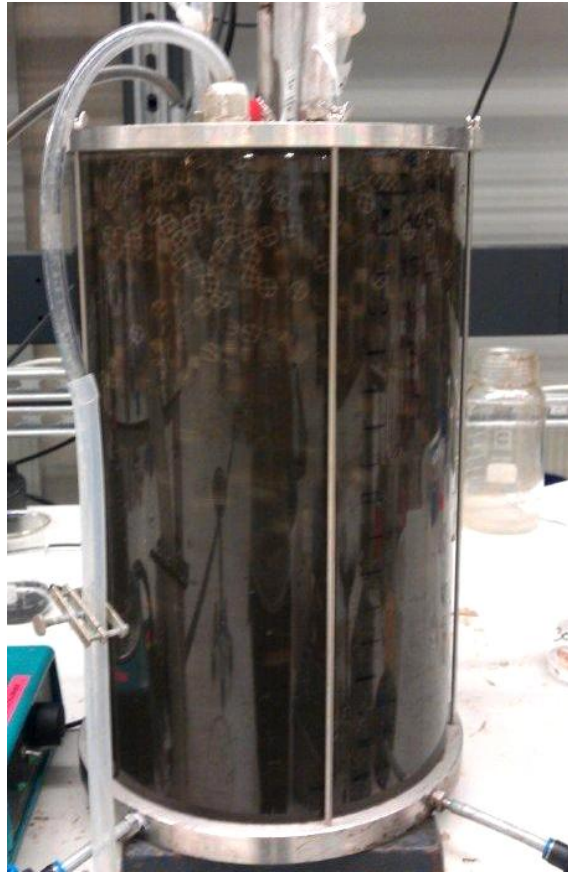
Figure 4.4 – Denitrification batch test with kaldnes carriers
