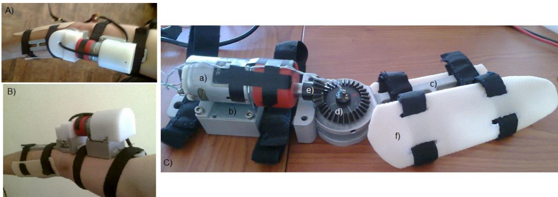
Figure 2.2 – Final state of the mechanical part of the SpastiMed device. A) Top View when attached to a subject arm. B) Side View when attached to a subject arm. C) View of the device without the white plastic protective covers. a) DC motor. b) arm metallic part. c) forearm metallic part. d) bigger conic gear. e) smaller conic gear. f) splint parts to help locking the device in position on top of an arm.
