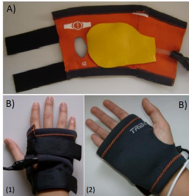
Figure 1.8 – Spasticity measurement device developed by Inês Clemente [16]. A) Inside view of the glove (plastic water sac inserted between the glove and the yellow tissue). B) Outside view ( (1) back of the hand (2) and palm of the hand) of the Glove when correctly strapped on an examiner's hand [16].
