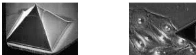
Figure 6. OLYMPUS OMCL TR-400-type silicon nitride tips. Images taken from OLYMPUS's catalogue. The image on the left is a tip's upper-side view. The image on the right is an image taken by the AFM's video camera where the cantilever's contact with the cell is represented.
