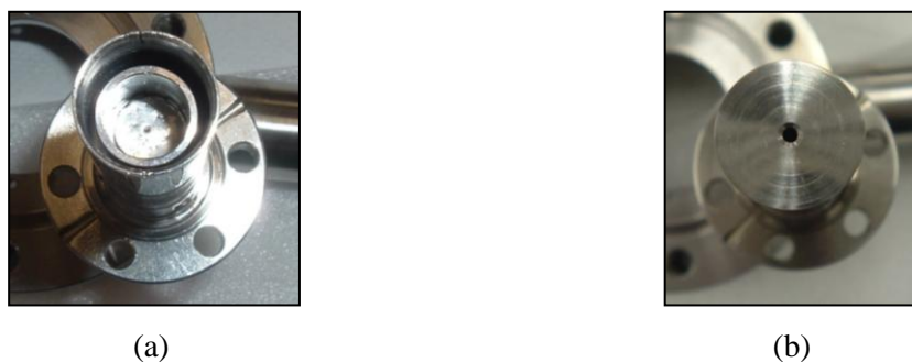
Figure 7.4. Faraday Cup components: (a) inner and outer cylindrical electrodes and (b) cap. Ceramics was used to isolate the collector from the ground.
