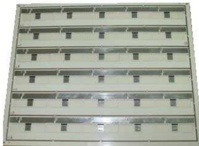
Figure 83 – Set of six PCBs that are the base for the HSUN sub-receivers.
