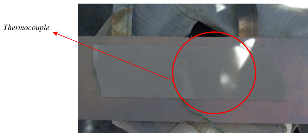
Figure 111 - Placement of the Thermocouple in the back rear surface of the solar cell n° 3 of the sub-receiver. To the acquisition of temperature by the thermocouple was made always in the same location, the thermocouple was fixed with thermal tape
