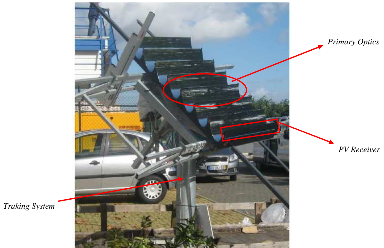
Figure 79 – HSUN module mounted on a 2-axes tracking system
