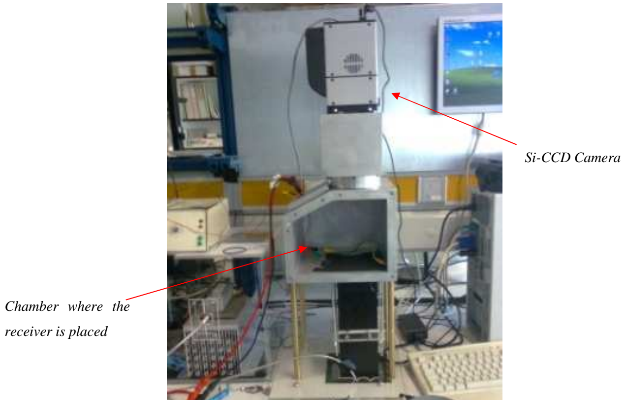
Figure 43 – Electroluminescence apparatus, located in the laboratory of the Faculty of Science, University of Lisbon (FCUL)
