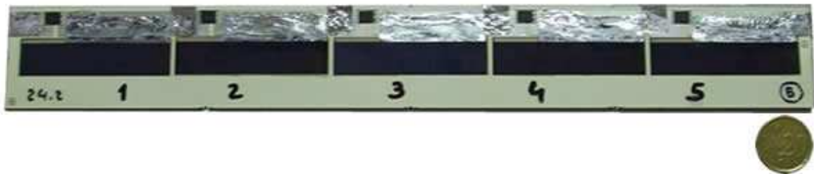
Figure 81 – Sub-receiver. When three of these sub-receivers are connected, a receiver is obtained.
