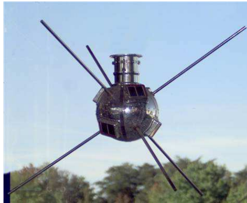
Figure 2.2 – Vanguard 1 was the fourth artificial satellite launched and the first to be solar power. It's the oldest satellite orbiting Earth, but there is no longer any communication with it. Source: http://nssdc.gsfc.nasa.gov/nmc/spacecraftDisplay.do?id=1958-002B
