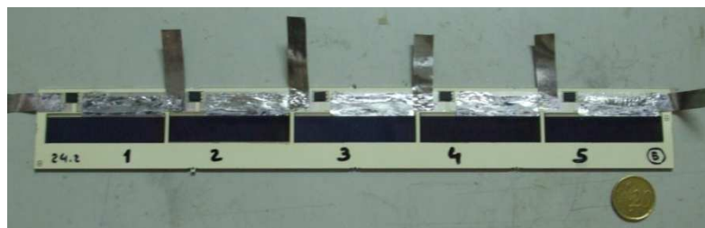
Figure 103 – Sub-receiver with the output ribbons soldered.
