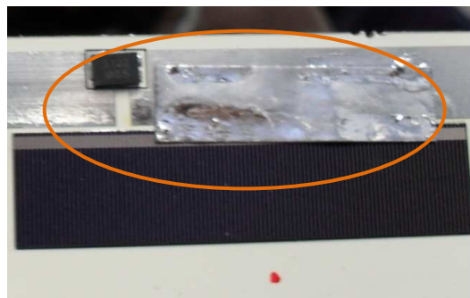
Figure 87 – Displacement of the ribbon from its specific position.
