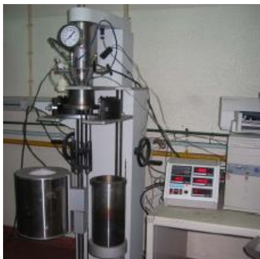
Figure 28. Stirred batch autoclave of 5 L from Parr Instruments of UTCAE-LNEG 183 .
