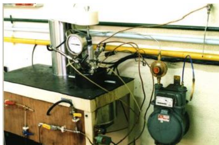
Figure 9. Stirred batch autoclave of 1 L from Parr Instruments of UTCAE-LNEG 175 .
