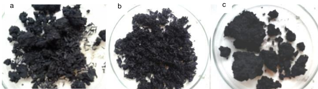
Figure 29. Crude chars obtained in the pyrolysis experiments (a: char 1, b: char 2; c: char 3).
