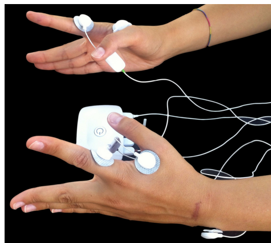
Figure 2: Contralateral acquisitions experimental setup: Bioplux research device, placement of two EMG sensors and ground.
