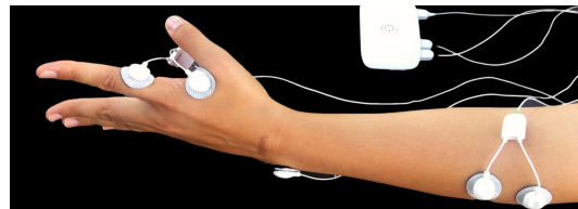
Figure 1: Ipsilateral acquisitions experimental setup for left member: Bioplux research device, placement of two EMG sensors and ground.
