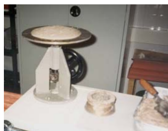
Figure 5 – Flow table consistency of the mortar
