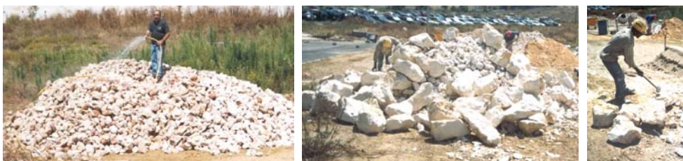
Figure 1 – Preparation of the stones used in the construction the experimental models
