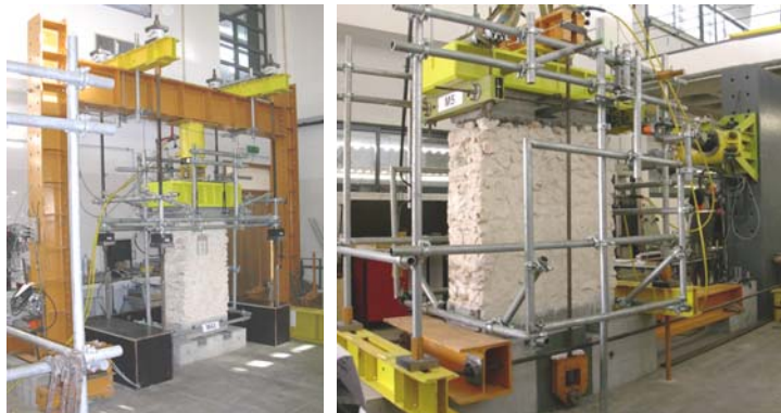
Figure 12 – Axial compression and shear-compression testing systems
