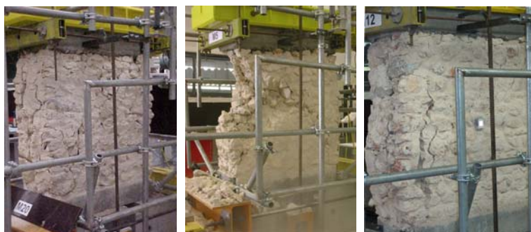
Figure 14 – Results of the three experimental testes under compression-shear loads
