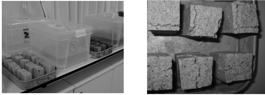
Fig. 4 – Sulphates resistance test: samples for immersion and general deterioration of the samples
