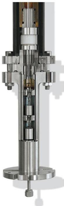
Figure 3.3. ISOSORP 2000 high-pressure magnetic-suspension balance (MSB) from Rubotherm GmbH (Bochum, Germany).
