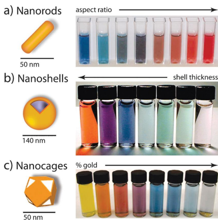
Figure 4. Gold nanoparticles commonly applied in biomedical applications. (a) Gold nanorods, (b) silica-gold core-shell nanoparticles, and (c) gold nanocages. The intense colour of these nanoparticles arises from the collective excitation of their conduction electrons, or surface plasmon resonance modes, which results in photon absorption at wavelengths which varies with (a) aspect ratio, (b) shell thickness, and/or (c) galvanic displacement by gold.
