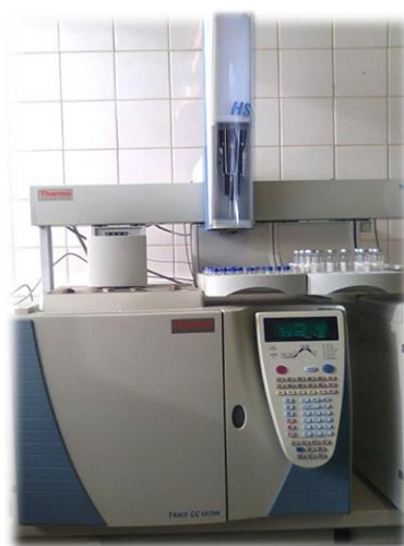
Figure 2.3 – Chromatograph Trace GC Ultra, with a TriPlus Autosampler headspace injector.
