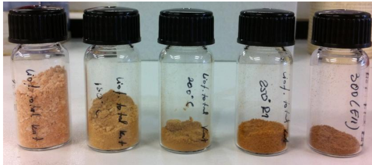
Figure 5.3 - Visual aspect of powders of GP hydrolysates obtained at different temperatures (from left to right: 150 °C; 180 °C; 200 °C; 250 °C; 300 °C) after lyophilisation.
