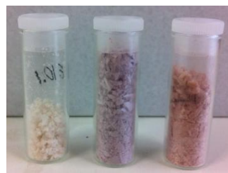
Figure 4.2 - Example of powders resulted from the lyophilisation.
