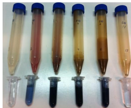
Figure 4.22 - Visual aspect of the liquid phase of hydrolysates collected during 150°C assay (above) and the same samples during colorimetric test to determine TPC (below).
