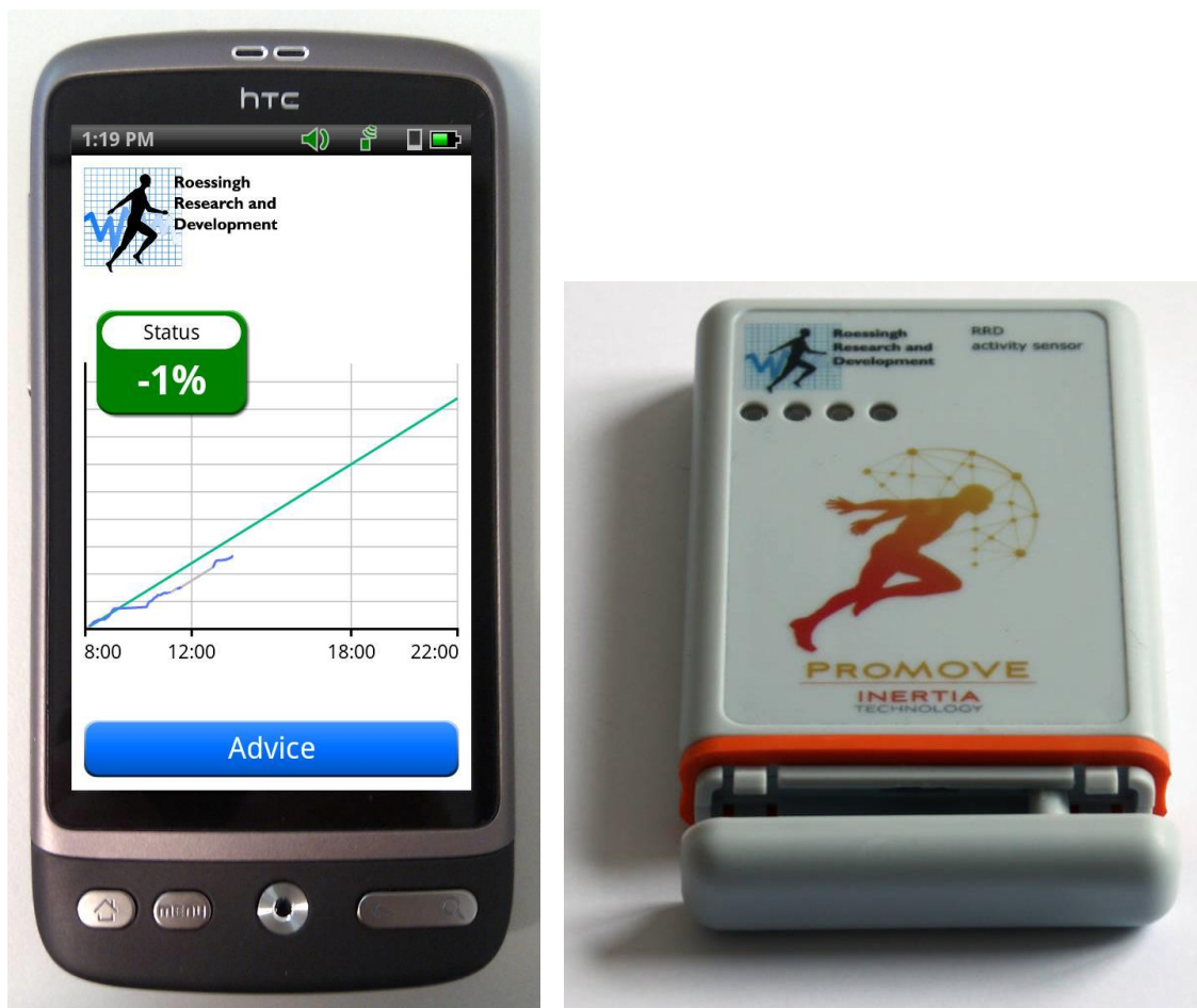
Figure 3 - Activity Coach consisting of a smartphone (left) and the sensor ProMove-3D (right).
