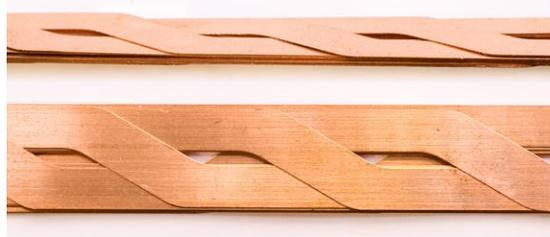
Figura 4.4 – Cabos de Roebel (condutores transpostos) (<http://www.gcsuperconductors.com/about-us/galleries/gcsgallery/hts-cable-and-weave-closeup>)
