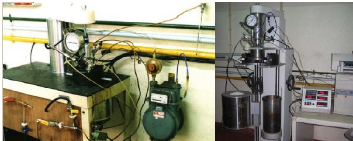
Figure 12. Stirred batch autoclaves of 1 and 5 litres from Parr Instruments used to perform the pyrolysis assays.
