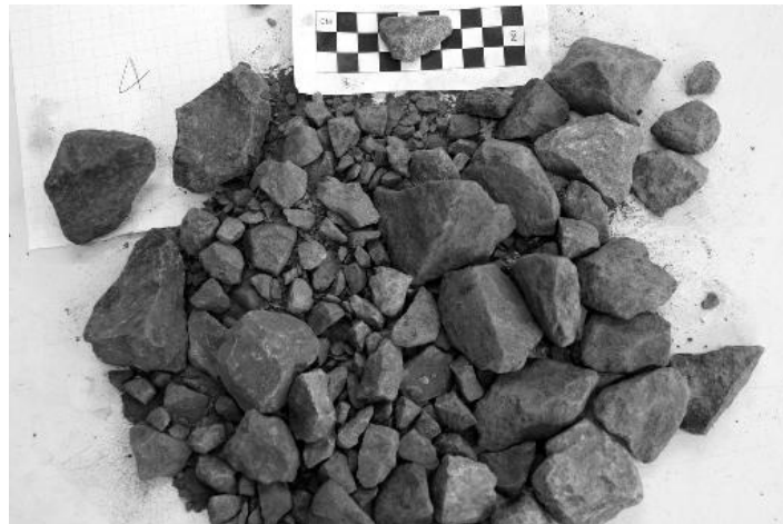
Figure 2.8: Photo of ballast sample taken from the track on top of the culvert
