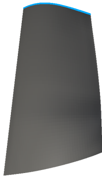
(a) Fan blade (tip gap in blue)
