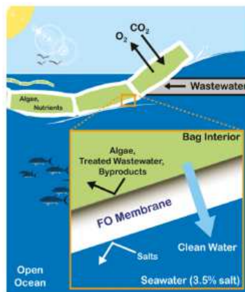
Figure 23- Schematic of the Offshore Membrane Enclosure for Growing Algae (OMEGA) system. Inset shows the permeation through and rejection by FO membrane in contact with the seawater. The top of the enclosure, which is in contact with atmosphere, contains specialized membranes that allow the passage of sunlight and the exchange of \text{CO}_2/\text{O}_2 to facilitate the algae photosynthesis (Hoover, et al., 2011)
