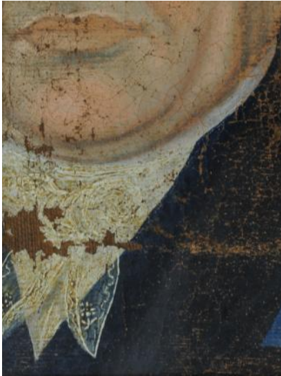
Figure 32: Initial efforts to document the distribution of the protrusions at the surface of the painting. Problems with discriminating lead soap protrusions from other surface defects was encountered, so that imaging did not provide exclusive evidence of lead soaps for the mapping desired.
