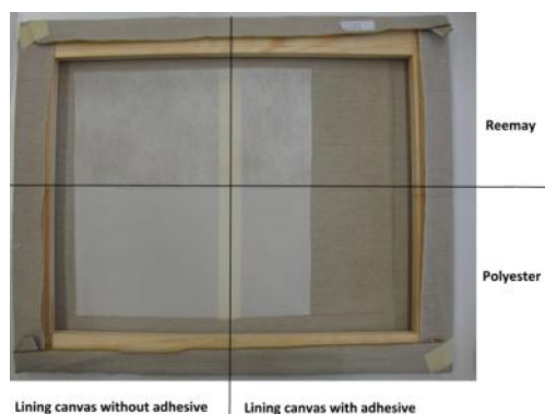
Figure 41: Lining canvas with adhesive (on one-half) and with the two interleafs. Interleafs had adhesive on both sides. On top of this, a piece of fabric was placed to simulate the "painting" to be lined.
