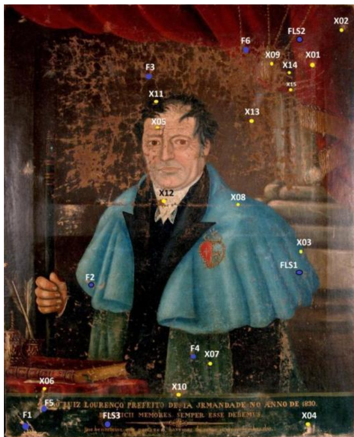
Figure 36: Areas sampled for mounting into cross-sections (X, signed with yellow dots) and for \mu -FTIR (F, marked with blue dots)
