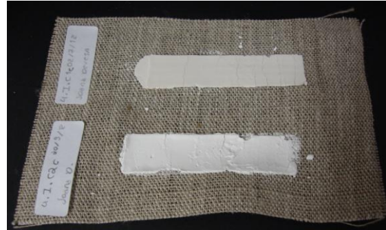
Figure 29: Isinglass filler. The largest deformation is associated with chalk nº2. The side of the canvas where chalk nº1 was applied was not deformed.
