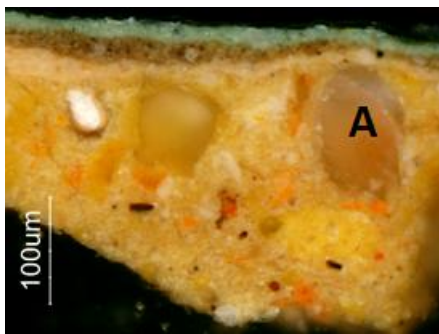
OM section X10: 200x mag. Vis. light - Polarized Light Legend: ○ lead carbonate ● red lead
