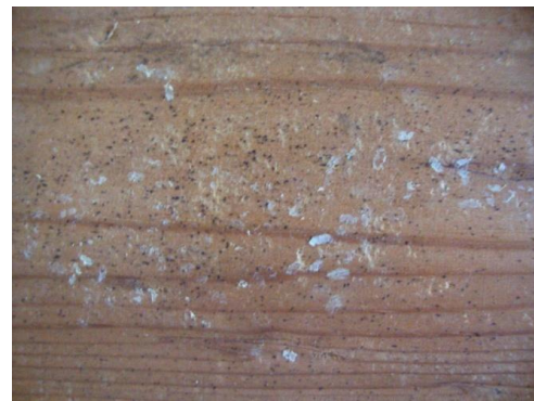
Figure 21: Signs of fungi and insect debris (carcasses) on the surface of the stretcher.
