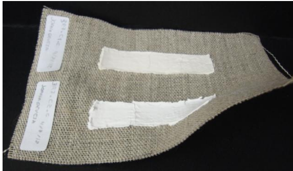
Figure 28: Rabbit ski glue filler on canvas. This was the filler that presented the greatest deformation upon drying.
