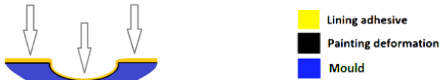
Figure 26: Diagram illustrating the concept of the system developed to remove the lining adhesive involving the creation of a solid mould to allow pressure needed during this procedure.
