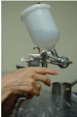
Figure 45: The spray gun used during the lining trial.
