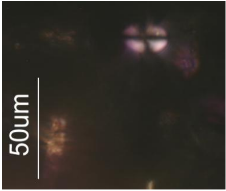
Figure 27: OM image from another area of the sample showing a centred extinction cross characteristic of starch under crossed polarized light [12] - total magnification 500x.
