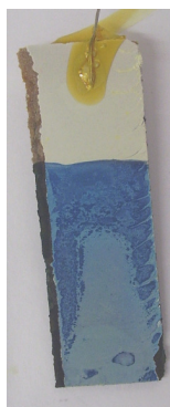
Figure 6.4 – Prussian Blue film electrochemically deposited over a TCO coated white board (white board electrode). The PB films are highly heterogeneous in all the electrode-substrates tested.
