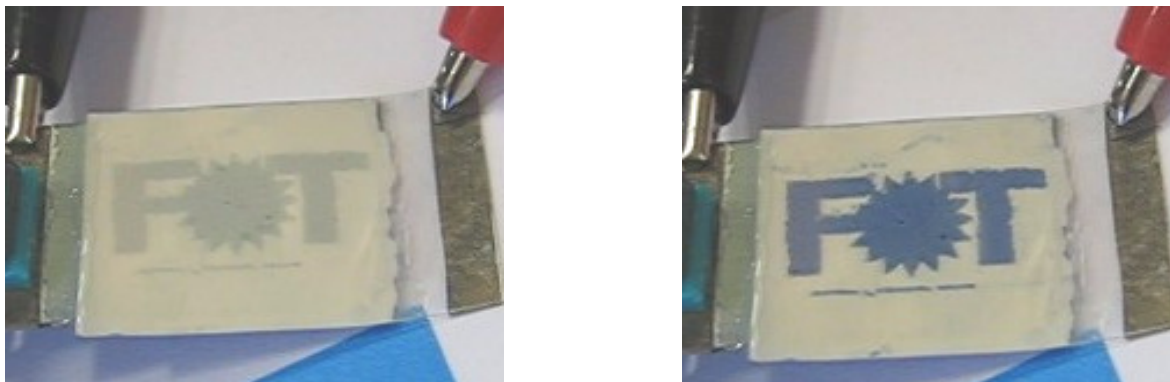
Figure 6.14 – Pictures of the bleached (left) and coloured (right) optical transition of an ECD based on PEDOT:PSS modified white board-electrode. Electrochromic device architecture: White board-electrode/PEDOT:PSS/white opaque electrolyte/PEDOT:PSS/ITO-PET.
