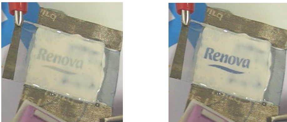
Figure 6.10 – Pictures of the bleached (left) and coloured (right) optical transition of an ECD based on PEDOT:PSS modified paper-electrode. Electrochromic device architecture: Paper-electrode/PEDOT:PSS/white opaque electrolyte/PEDOT:PSS/ITO-PET, where the primary electrode is the PET-ITO.
