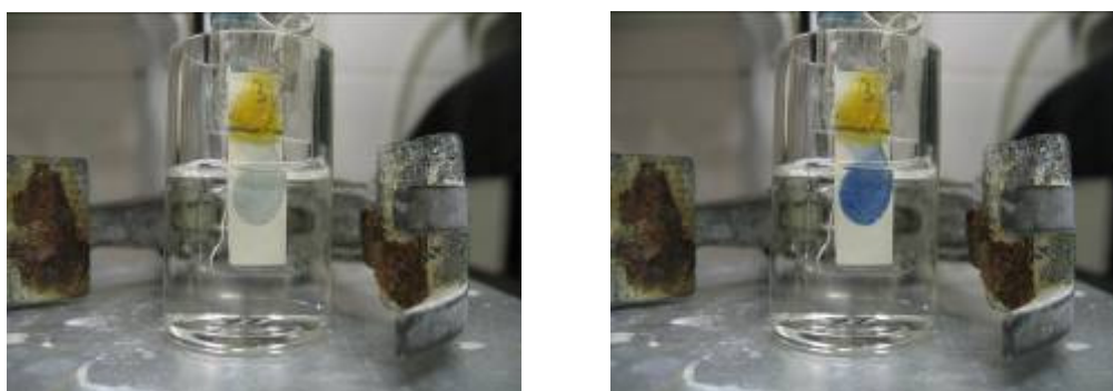
Figure 6.7 – Images of the optical transition of PEDOT:PSS layer deposited over the paper-electrode by electrochemical oxidation (left) and electrochemical reduction(right). See experimental details in Table 6.6.
