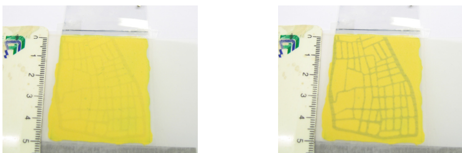
Figure 6.11 - Pictures of the bleached (left) and coloured (right) optical transition of an ECD based on PEDOT:PSS modified paper-electrode. Electrochromic device architecture: Paper-electrode/PEDOT:PSS/yellow opaque electrolyte/PEDOT:PSS/ITO-PET, where the primary electrode is the paper-electrode.
