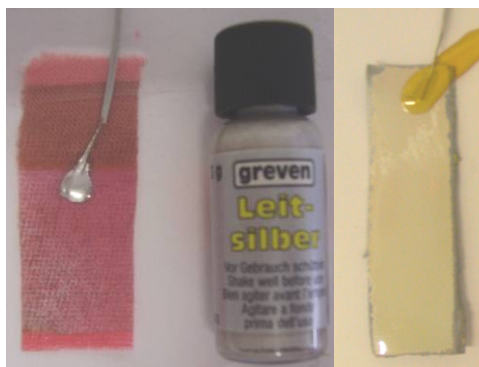
Figure 6.3 – Substrate-electrode preparation with an electrical contact. Copper electrical wires were connected to the TCO layer through conductive silver glue (left, textile-electrode sample). After the silver glue is dried epoxy glue is used to seal and give structure to the contact between electrical wire and the substrate-electrode (right, white board-electrode sample).
