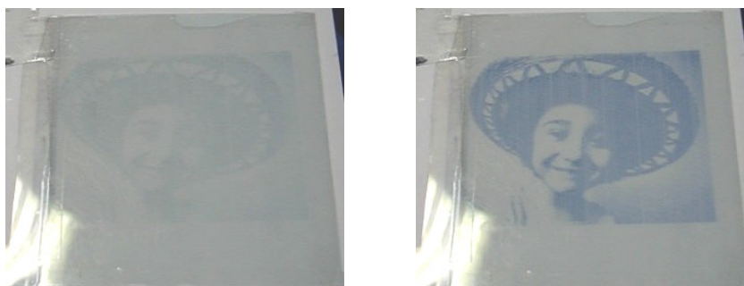
Figure 7.8 - Ink-jet printed ECD (7 x 7 cm) showing the coloured state (left) and bleached state (right)
