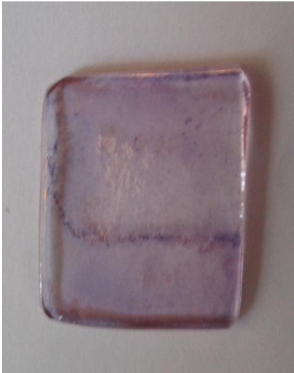
Figure 3. Clear glass sample using 700 °C; 6bl; Au 0.002 g/ml.
