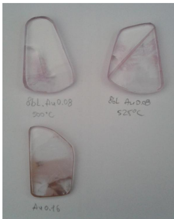
Figure 2. Picture of clear glass samples thermal treated at 500 °C and 525 °C for 1 hour; 8bl; Au 0.002 g/ml, 0.004 g/ml.
