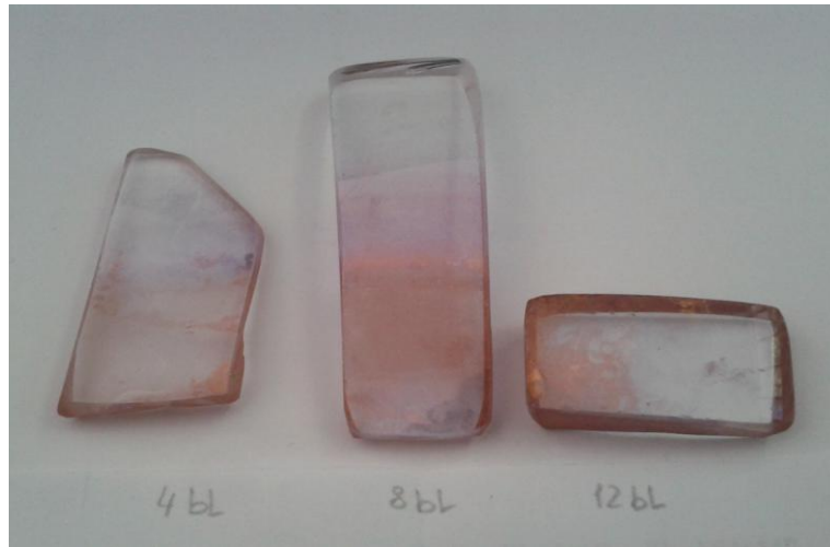
Figure 9a. Picture of clear glass samples using 600 °C for 1 hour; 4bl, 8bl, 12bl; Au 0.004 g/ml.
