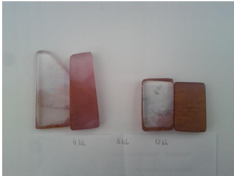
Figure 7a. Picture of clear glass and samples with texture using 600 °C for 1 hour; 4bl, 12bl; Au 0.004 g/ml.
