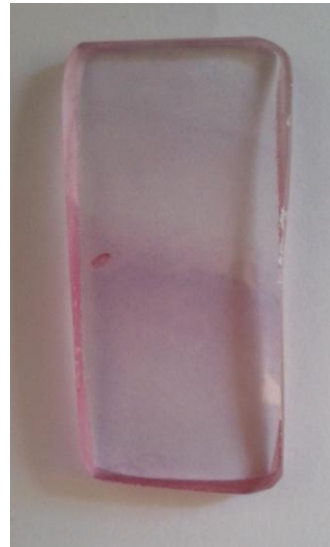
Figure 4. Clear glass sample using 600 °C; 6bl; Au 0.002 g/ml.
