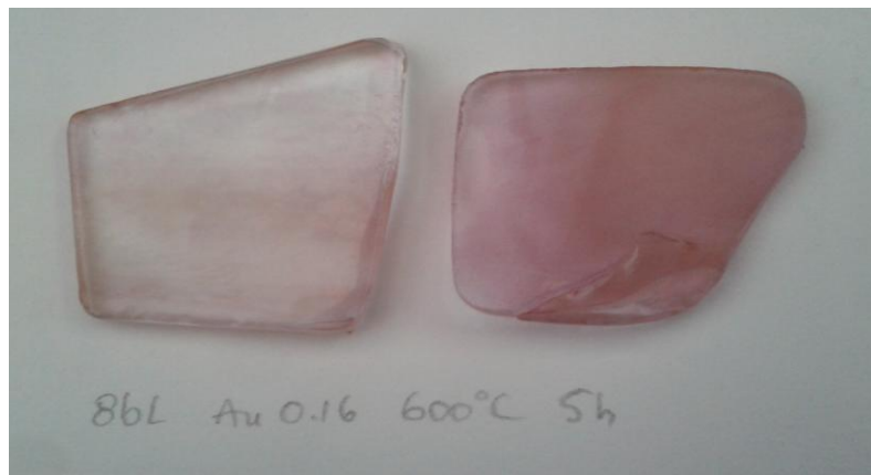
Figure 5. Picture of clear glass sample and sample with texture using 600 °C for 5 hours; 8bl; Au 0.004 g/ml.
