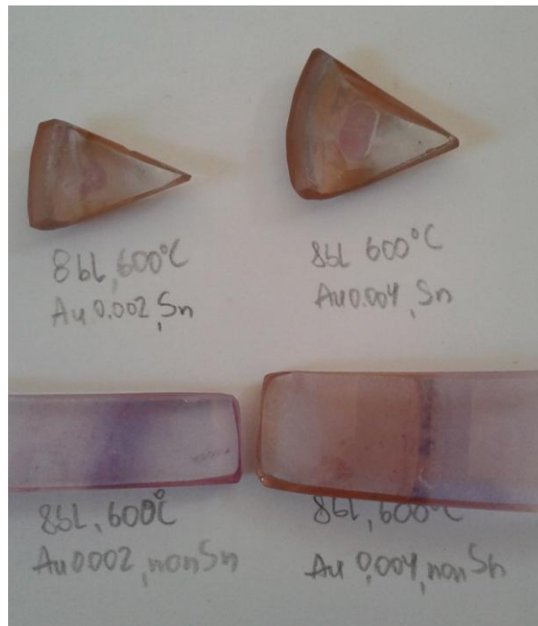
Figure 10a. Clear glass samples using 600 °C; 8bl; Au 0.002 g/ml, 0.004 g/ml; two of the samples have Sn.
