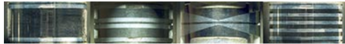
Figura 11. Diferentes Formatos de Cabeças 56 : Full Track Mono, Half Track Mono, Half Track Amateur Stereo (Mariposa) & Quarter Track.
