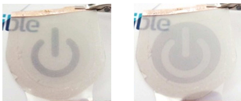
Figure 118: Paper-electrode device with \text{WO}_3 inkjet printed as electrochromic material.
