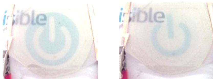
Figure 120: Paper-electrode device with PB inkjet printed as electrochromic material.
