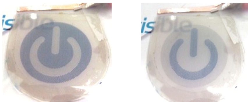
Figure 117: Paper-electrode device with PEDOT:PSS inkjet printed as electrochromic material.
