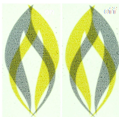
Figure 111: Solid-state electrochromic device obtained with printed \text{V}_2\text{O}_5 ink.
