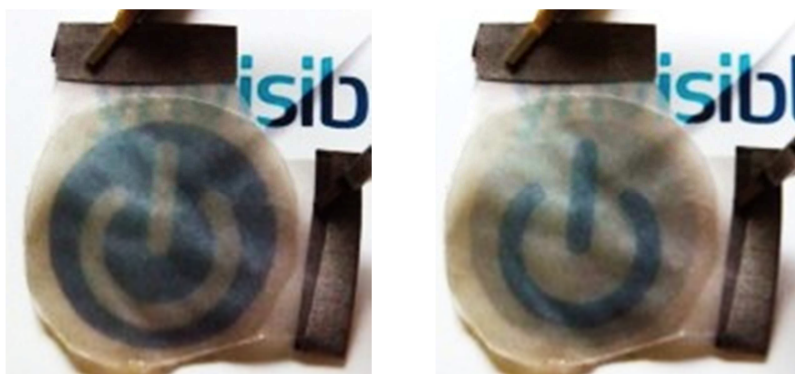
Figure 115: Images of a working device build with architecture 4 (Drafting paper / Drafting paper). This was not the device characterized in this section.
