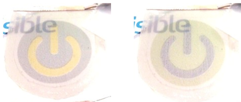
Figure 119: Paper-electrode device with \text{V}_2\text{O}_5 inkjet printed as electrochromic material.
