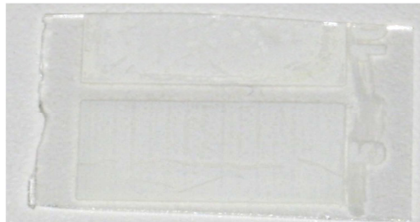
Figure 36: Deposition of ITO via sol-gel on glass using inkjet printing.
