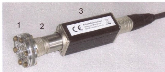
Figure 9.6: new condenser microphone.
