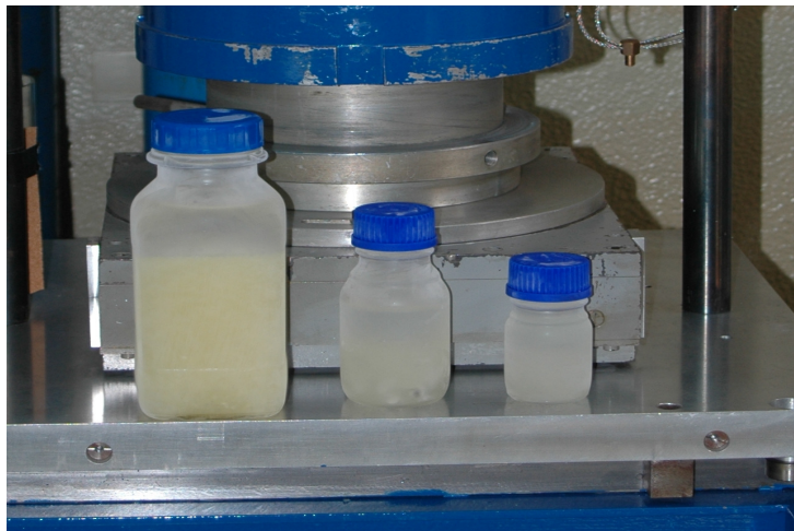
Figure 3.6: three sizes of SDDs: from left to right, 900 ml, 150 ml and 80 ml.
