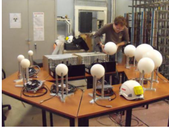
Figure 7.26: characterization of the GESA measurement site with Bonner spheres.
