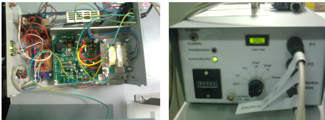
Figure 9.3: (L>R) recompression electronics for the BDC; and the system in operation.
