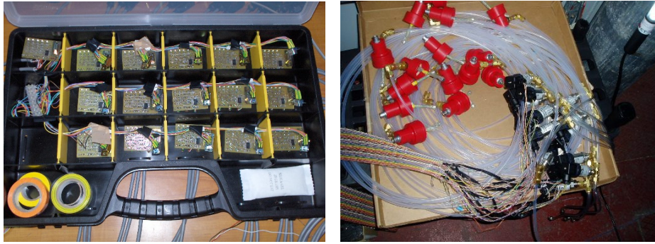
Figure 7.5: DAQ system (L > R) preamplifier “core”, SDD capping & pressure transducers.
