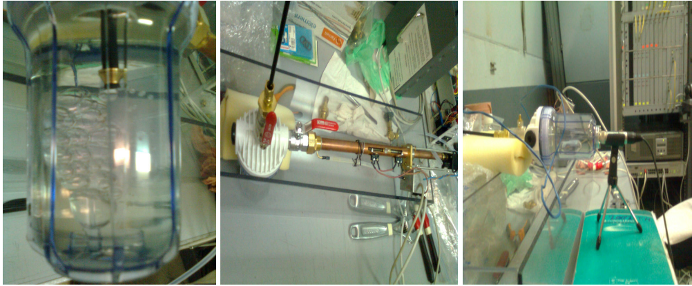
Figure 9.8: (L>R) Freon injection, BDC coupling to piston and ultrasound microphone adjustment.
