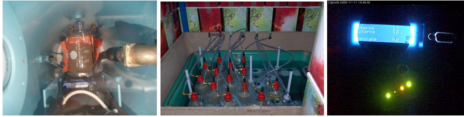
Figure 7.7: (L > R) SDD freon injection, SDDs being installed, and remote temperature monitoring.
